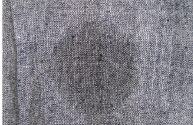
This fabric is made with both black and white yarns. The black yarns have bled into the white ones, causing permanent damage.
